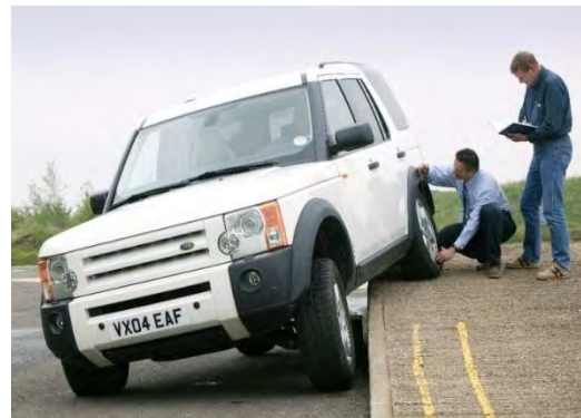
Articulation ramp (How high can one wheel get with the other 3 still in contact with the floor?)
