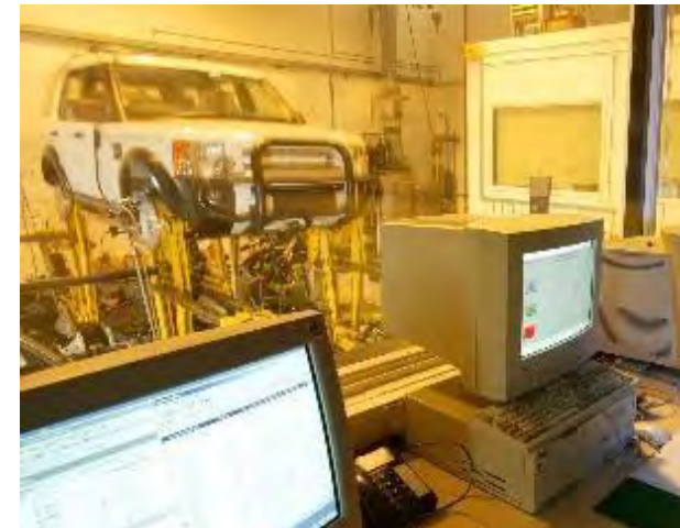
Hydraulic rig test (durability)
