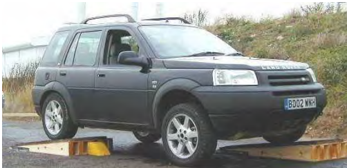
Articulated traction test (2 wheels just contacting floor –can the vehicle drive forward?)
